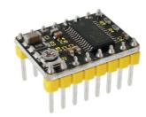
The DRV8825 features adjustable current limiting, over-current and over -temperature protection, and six microstep resolutions (down to 1/32-step) It operates from 8.2-45V and can deliver up to approximately 1.5A per phase without a heat sink or forced air flow (rated for up to 2.2 A per coil with sufficient additional cooling).
